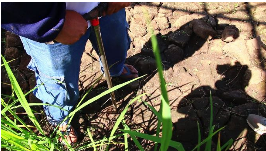
Use an auger or pipe that is similar diameter to the tensiometer
