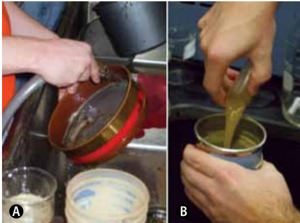
**Figure I.** Rinsing material collected on a 38  $\mu\text{m}$  sieve (A) and collecting nematodes after centrifugation with a 25  $\mu\text{m}$  sieve (B).
