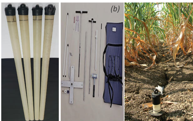
Fig. 6: (a) Porous access tubes, (b) accessories for installation of the tubes in field and (c) a tube properly installed in field.
