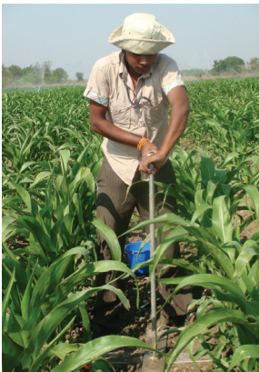
Fig. 7(a) Installation of tubes in field and (b) distribution of porous tube for soil moisture data recording using soil moisture profile probe in a drought trial field.
